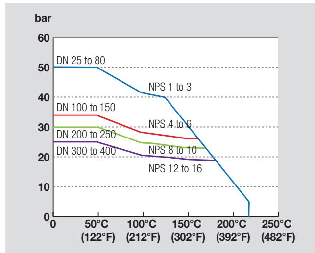
Soft R-PTFE seat ratings are based on differential pressure with the ball in the fully closed position and refer only to the seats. The maximum allowed differential pressure can be further reduced if the maximum allowed working pressure, based on body material and pressure class of the valve, is lower than the maximum allowed differential pressure.
