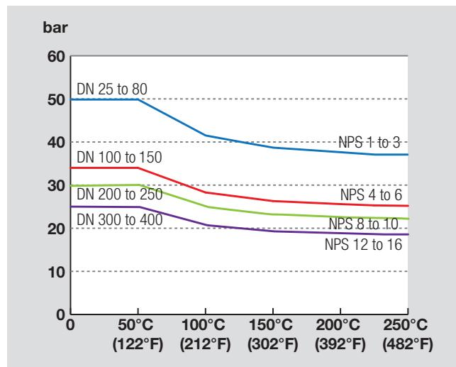
Please note that the maximum allowed differential pressure can be further reduced if the maximum allowed working pressure, based on body material and pressure class of the valve, is lower than the maximum allowed differential pressure.
